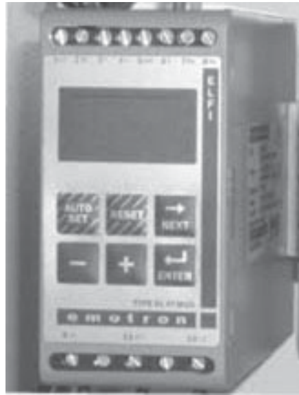
Figure 9 Power Monitor Terminals 3 and 4 for analog output of 4-20mA signal proportional to shaft horsepower
